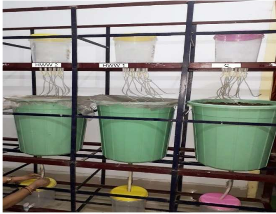
Fig. 2: Vermifiltration unit assembled on the movable iron rack
